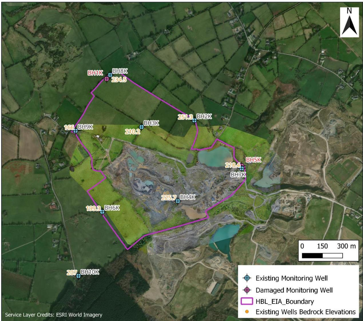
**Figure 5-15 - HBL Monitoring Wells and Bedrock Elevations (orange text, mAOD)**
